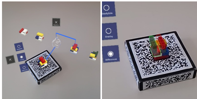
Fig. 1. Prototype showing the concept of Tangible Version Control [18]. Left: a timeline of virtual versions can be explored by moving the physical artifact. Contextual information about ongoing comparisons and between physical and virtual content are marked by blue highlights. Right: comparisons between two versions are displayed directly on the physical artifact. In the image, the Differences-mode is used, in which differing parts of the physical object are highlighted by color-coded outlines.
